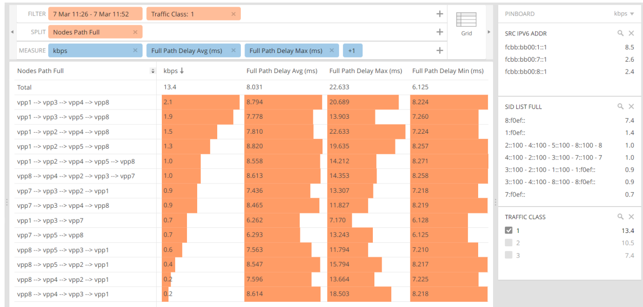
Figure 4.2: Turnilo visualization: bandwidth and avg/max/min delay for customer 1’s paths in the network (filtering for tc=1).
